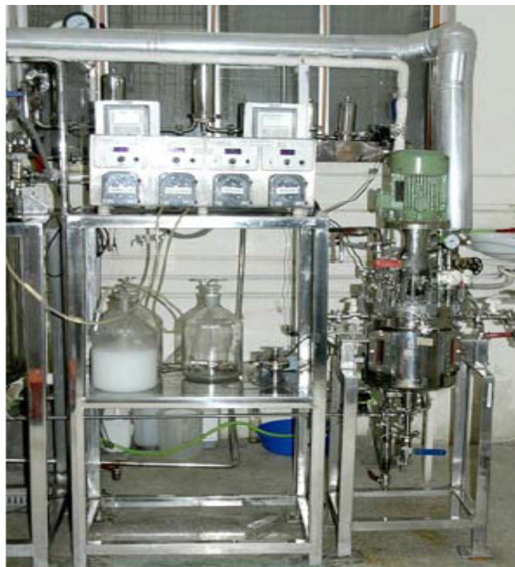
Fig. 4.2 : The 14 L SS fermentor used for CGTase production
