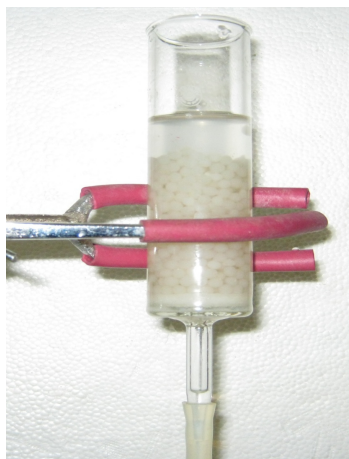
Fig. 6.5 : Packed bed reactor with immobilized cells of E. aurantiacum for production of CD
